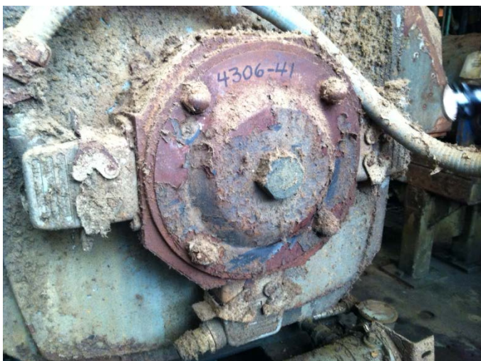
Figure 1: Magnetic encoders operate effectively even when covered with dust and oil.
